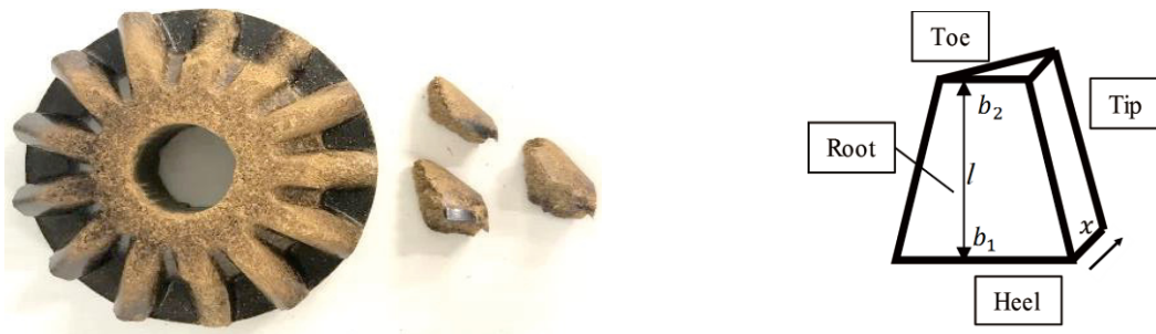
Fig. 12 Fracture surface of bamboo fiber gear
