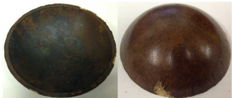
Fig. 13 Bamboo hemisphere shell shape product with improved method
