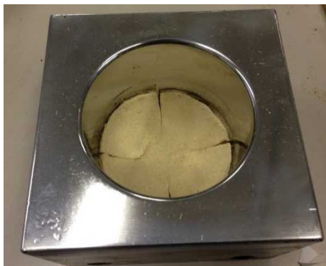
Fig. 12 Bamboo fiber plane sheet after fitting in mold die
