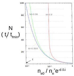
ne\*: critical electron density at the time of just starting breakdown
