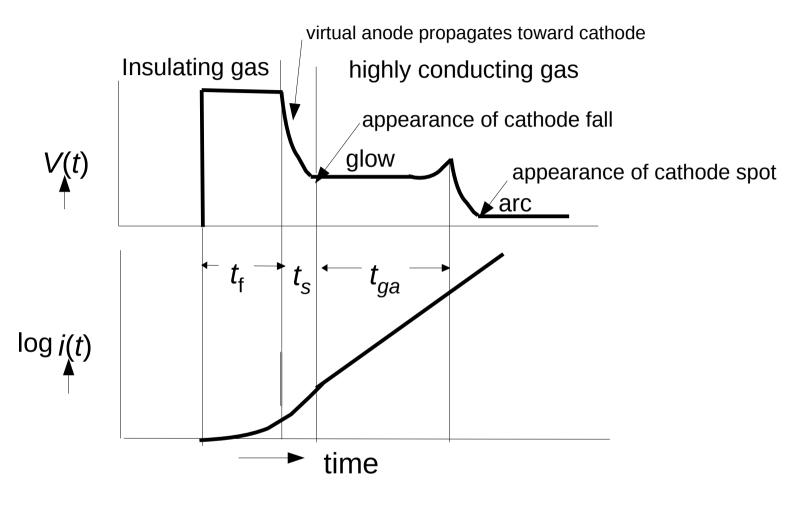
$t_f$ : formative time lag, time to the just starting breakdown by applying step voltage.
