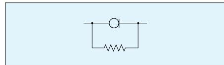
Compensative resistor is not necessary if the current value is less than 1 mA.
