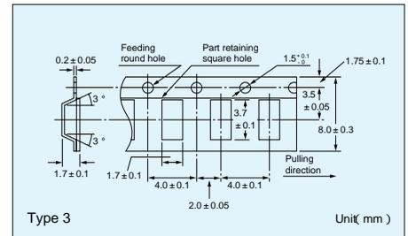
\*In principal elements are set with cathode side on the round hole side.
