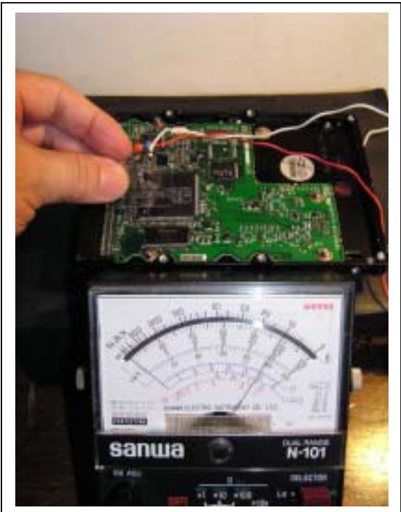
Look for leakage between adjacent leads using a multimeter
