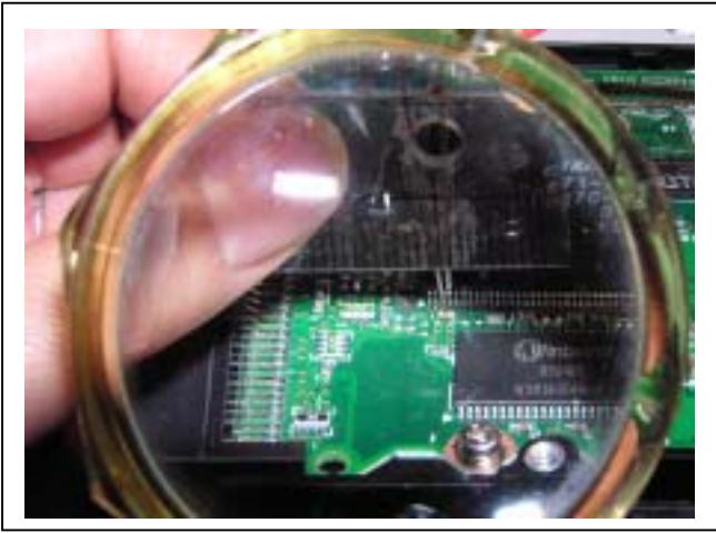
Probing adjacent leads by a hand-made jig under magnifying glass
