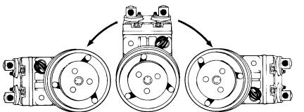
NOTE: CCI recommends that when positioning compressor at full 90° horizontal, suction side should be on "top".
