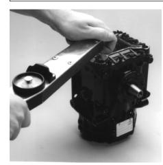
3. Install the baseplate and bolts. Tighten baseplate bolts to 10-16 ft. Ibs. (13.6-21.7 N-m) in sequence given on page 15 using a torque wrench.
