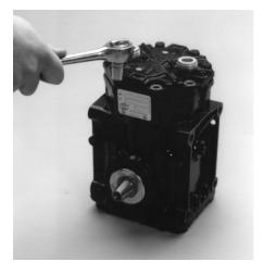
2. Remove the remaining screws in the head and remove the valve plate and head from the cylinder by prying or tapping under the ears which extend from the valve plate. If the head and valve plate adhere, hold the head and tap the valve plate ears away from the head with a soft hammer. Do not hit or tap the head to separate the head and valve plate because damage to the head may result.
