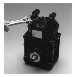
1. Remove the screws from flanged type service valves. Note that these four screws are longer than the remaining head screws. If the valves are of the Rotalock type or Tube 'O' type, remove by loosening the hex nuts which are a part of the valve assembly.
