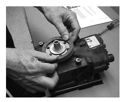
8. Install felt ring dust shield, placing it around the seal plate and tight against the compressor housing.
