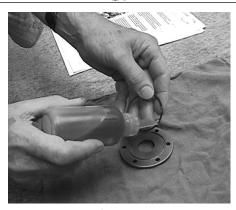
2. Apply clean refrigerant oil to the seal plate "O" ring and place the ring into the seal plate "O" ring groove. Invert the plate and observe that the "O" ring remains in place.
