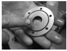
3. Place a few drops of clean refrigerant oil on the face of the seal plate between the "O" ring and the inside diameter and with a clean finger spread the oil into a thin film. It is important that the surface not be over oiled and that there is no oil between the "O" ring groove and the outside diameter of the seal plate.
