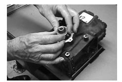
5. Prior to installation, check the seal assembly to make sure that the carbon seal ring is right side up (narrow polished band up), and confirm that the carbon rings notches are aligned with the drive tabs in the metal seal retainer. Lightly place the seal assembly (carbon ring side up) onto the oiled crankshaft.
