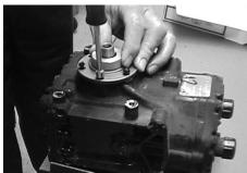
6. Insert the alignment tool into the seal plate and lightly place the plate's polished face into contact with the seal assembly. With a uniform downward motion, use the alignment tool to push the seal plate into contact with
