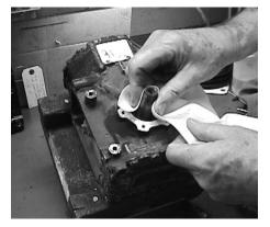
1. Use a clean, lint free shop cloth to wipe the crankshaft clean. Note: At this time the front main bearing is exposed, therefore care must be taken to prevent dirt or any type of contamination from falling into it.
