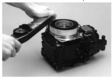
2. Mount and center the coil bracket. Tighten the four clutch mounting bolts using a torque wrench to 13-19 ft. lbs. (17.6-25.8 N-m). NOTE: Only use bolts that have a loctite patch on the threads.
