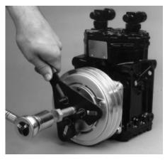
2. Install clutch removal bolt into the clutch. Using the adjustable spanner wrench to hold the clutch pulley in place, tighten the clutch bolt until the clutch pulley is forced free.
