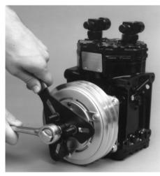
1. Remove the clutch center bolt and washer using the adjustable spanner wrench to hold the clutch pulley.
