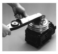
4. Install and tighten the clutch center bolt and washer using a torque wrench to 20-25 ft. lbs. (27.1-33.9 N-m).
