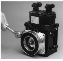
3. Remove the clutch mounting bolts.
