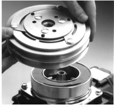
3. Place clutch pulley over shaft making sure to align the key way over the shaft key.
